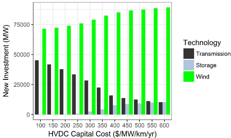
**Figure 13 Transmission Cost Sensitivity Analysis**
