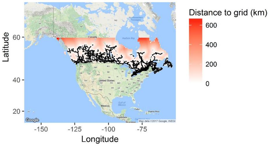
Figure 4 – Distance of MERRA Grid Cells to Existing Transmission Grid
