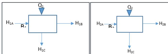
The savings in heating requirement – which is the net of  $Q_1$  and  $Q_2$  – amounts to the difference in fuel costs (OPEX) between the two boilers.
